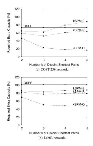
Fig. 2. Impact of multi-path routing and load balancing on the backup capacity of SPMs.
