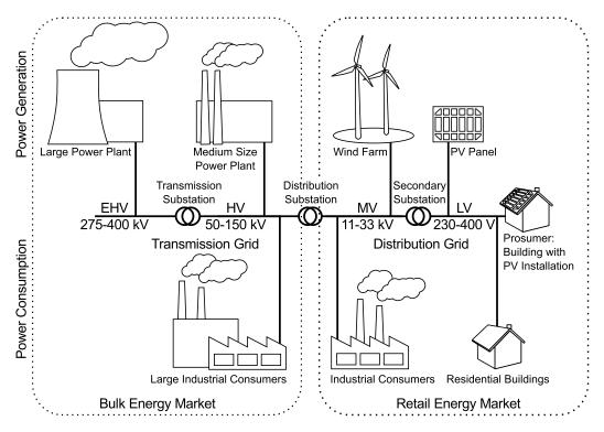
Fig. 1. The structure of a typical power grid including the general boundaries of the electrical energy market. Power is generated at the top, transfered over the transmission and distribution grid, and consumed at the bottom. Prosumers are positioned in-between the generation and consumption domain as they are part of both domains. Voltage levels decrease from left to right, i.e., from EHV level to LV level.
